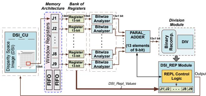
Fig. 6: Hardware architecture for the CA 1 Processing Unit.
