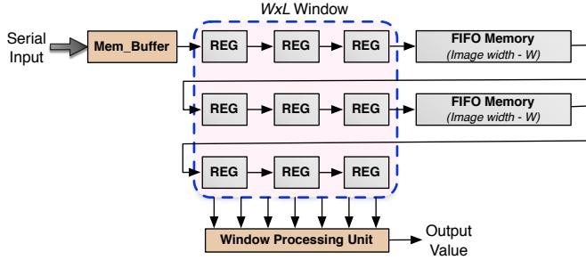
Fig. 7: Memory architecture for CA 1 Processing Unit.
