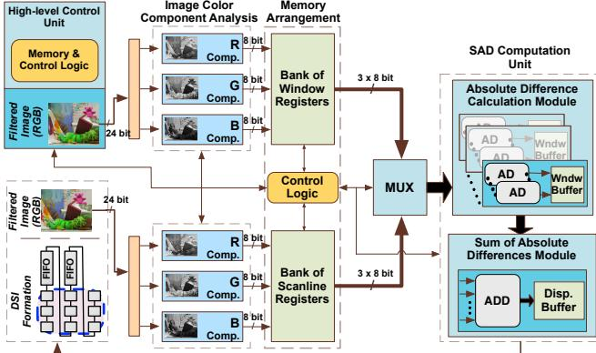
Fig. 5: DSI Creation Unit (DSI\_CU) architecture.
