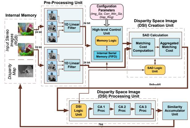
Fig. 3: Hardware architecture of the proposed real-time stereo vision system.
