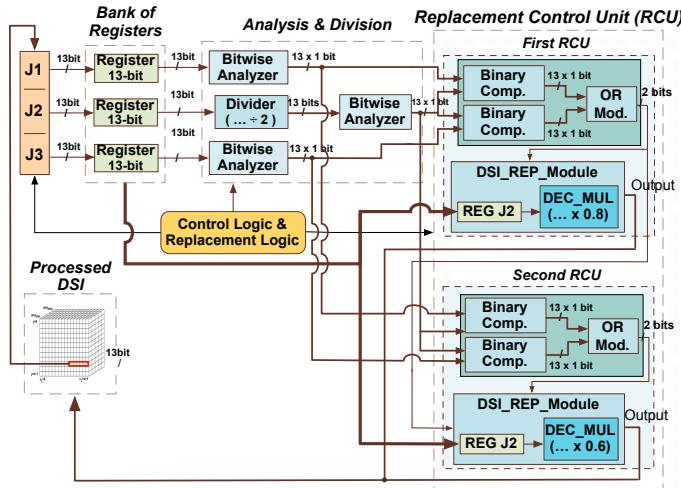
Fig. 8: Hardware architecture for the CA 2 Processing Unit.
