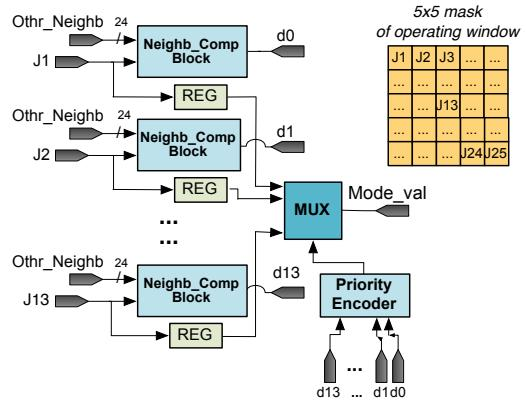
Fig. 12: Hardware architecture for the ModeFq\_Blk sub-module.
