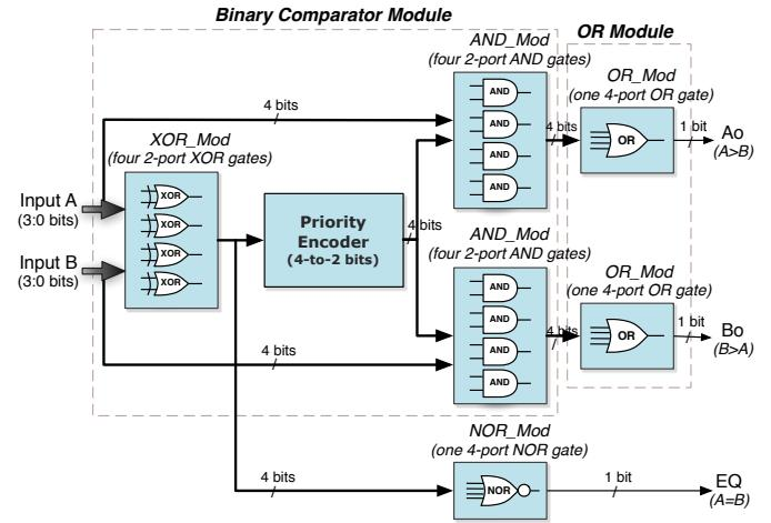
Fig. 10: The implemented binary comparator.
