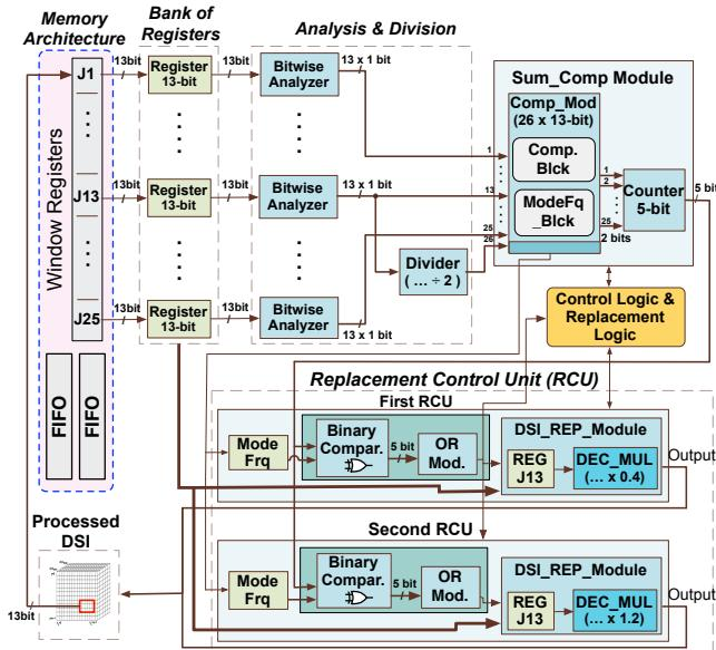
Fig. 11: Hardware architecture for the CA 3 Processing Unit.
