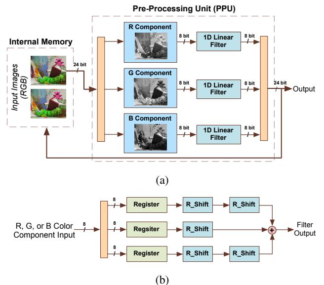
Fig. 4: (a) Pre-Processing Unit (PPU), and (b) one-dimensional linear pre-processing filter architecture.
