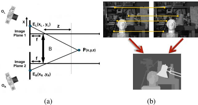
Fig. 1: (a) Stereo vision camera setup, and (b) the determination of corresponding scene points and the creation of the disparity map.
