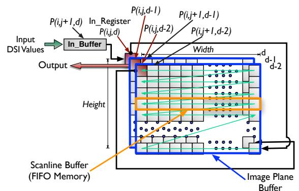
Fig. 9: Hardware architecture of the DSI Memory Block.
