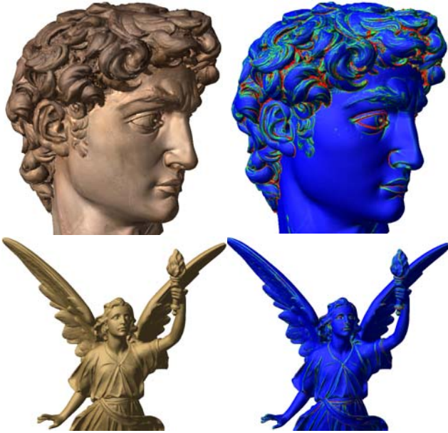
Figure 16. Results of applying normal computation and splot estimation; and curvature stream operators to raw point cloud data sets. The left column shows the high-quality normal estimation and on the right the qualitative (RMS) curvature strength is color coded.
