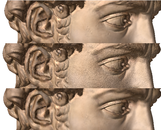
Figure 8. Original smooth surface (top); random noise of 0.05% of diagonal length added to each coordinate (middle); and smoothed model using our stream-process fairing operator (bottom).
