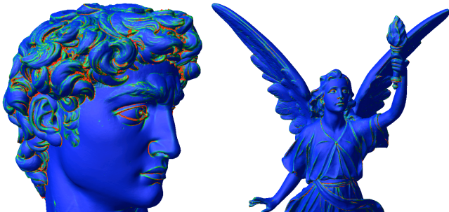
Figure 7. Results of applying normal computation, splat estimation and curvature stream operators to raw point cloud data sets. The images show the high-quality normal estimation and the color coded qualitative (RMS) curvature strength.
