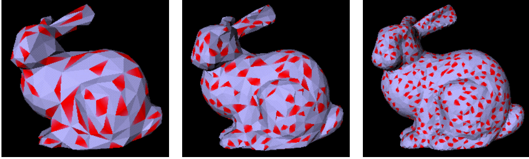
FIGURE 2. Batches of vertex split refinement operations of three different mesh updates (not consecutive in this example). The two triangles inserted by a vertex split are highlighted in each image.
