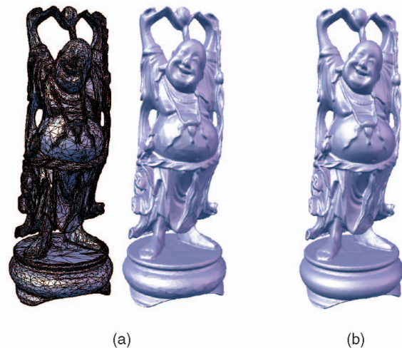
Fig. 17. Example of simplification based on shading tolerance. (a) Tolerated angular normal direction deviation is \varphi = 15^\circ , rendered 66 percent or 66,024 out of 100,000 faces. (b) The corresponding full resolution mesh.
