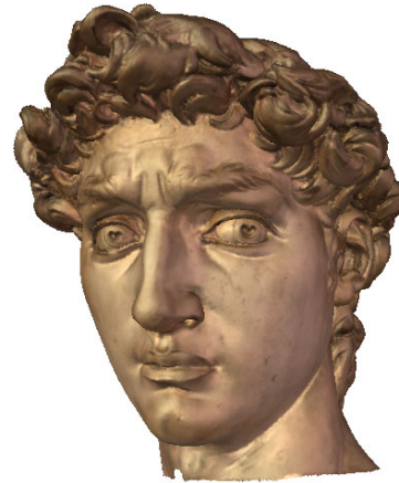
FIGURE 1. The head of Michelangelo’s David statue rendered with \tau=16 pixels screen tolerance, at 1/4 of the full resolution (510827 out of 2000606 points).
