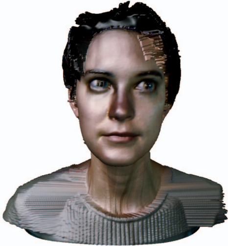
Fig. 1. Female head model at \tau = 1 pixels screen tolerance (rendered 113,012 out of 302,948 points at 2,647,209 splats per second).
