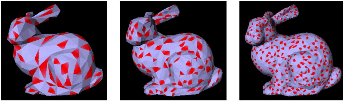
Fig. 3. Batches of edge collapses.
