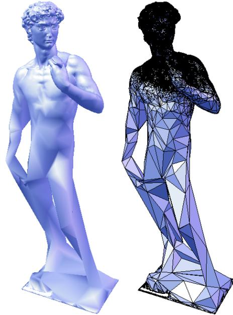
Figure 1: A model of Michaelangelo’s David statue, comprising over 8.25 million polygons. The model is shown as simplified with XFastMesh. The full-quality (within view frustum) smooth-shaded model is shown on the left, and the wire-framed, flat-shaded image on the right is shown to display the simplification. The view frustum is focused on the head and upper body.
