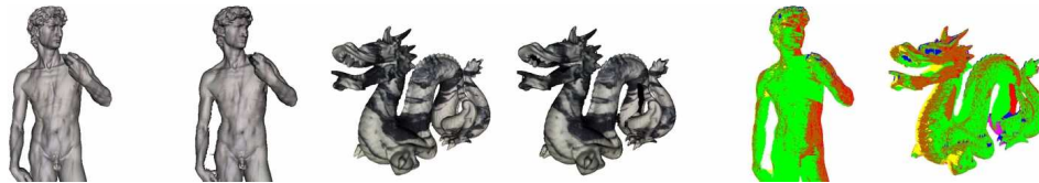
Fig. 19. Static DMesh rendering of complex polygonal objects. Left image shows the actual polygonal object and the right image shows the weighted blending of multiple textured depth-meshes. Various blending combinations of different depth-meshes are shown on the far right by different shading (pseudo colors), darkest shade (orange-brown) denotes two or more overlapping depth-meshes.
