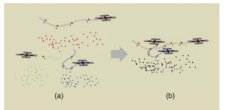
Figure 7. (a) The local-navigation module (running on board) estimates the pose of each MAV independently for each platform. (b) The global-navigation module (offboard) recognizes path intersections and uses them to express the MAVs' poses in the same, global coordinate frame and to reduce drift.
