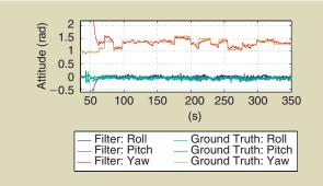
Figure 14. A comparison between EKF-based attitude estimate (filter: roll, pitch, yaw) and GPS-IMU based estimates from the AscTec internal state estimator (ground truth: roll, pitch, yaw) during a 5-min interval of time.
