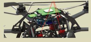
Figure 4. The computer-aided design (CAD) model illustrating the vibration damping between the two parts of the frame: the motors and the landing gear are connected to the outer frame, and the inner frame to the IMU, battery, and payload. The silicon dampers are highlighted in red.
