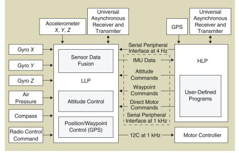
**Figure 3.** The electronic architecture: all sensors, except the GPS, are connected to the LLP, which communicates via I2C with the motor controllers and via the serial peripheral interface with the HLP. For this article, position control and state estimation for local navigation are implemented in the "user-defined programs" section of the HLP (see Figure 8). The position (waypoint) controller on the LLP is not used here since we work in GPS-denied environments.
