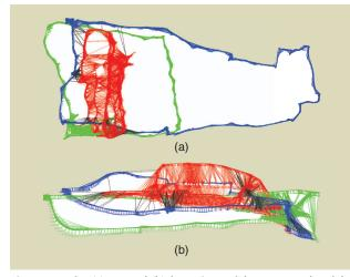
**Figure 18.** The (a) top and (b) front views of the pose graphs of the three flight trajectories in Figure 17 after map merging and global bundle adjustment. The black lines show the loop closures between the three submaps.
