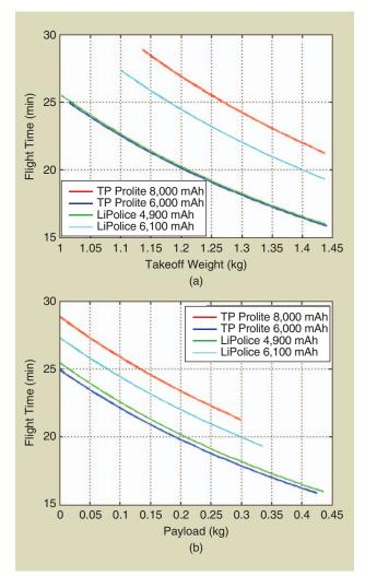
Figure 6. The calculated flight time is plotted versus (a) takeoff weight and (b) payload. The estimated flight time for a given payload with different batteries is shown. Thunder Power (TP) and LiPolice are LiPo battery manufacturers.
