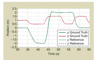
Figure 11. The plot shows the commanded reference trajectory and the measured ground truth.
