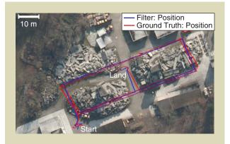
**Figure 15.** After a short initialization phase at the start, visionbased navigation (blue) was switched on for successful completion of a more than 350-m-long trajectory, until battery limitations necessitated landing. The comparison of the estimated trajectory with the GPS ground truth (red) indicates a very low position and yaw drift of the real-time onboard visual odometry.
