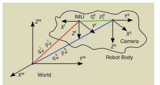
**Figure 9.** A setup depicting the robot body with its sensors with respect to a world reference frame. The system state vector is  $X = \{p_w^i v_w^i q_w^i b_w b_a \lambda p_i^s q_i^s\}$ , whereas  $p_w^s$  and  $q_w^s$  denote the robot's sensor measurements in (a possibly scaled) position and attitude, respectively, in a world frame.
