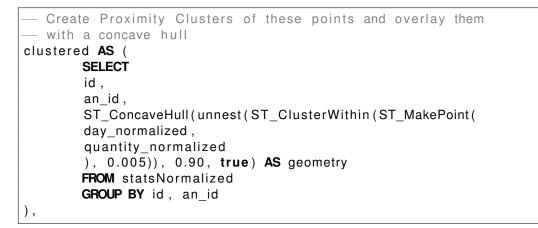
Figure 38: Cluster and apply concave hull to normalized point values
