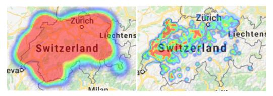
Figure 27: Heat Map with point scaling relative to map viewport (left) vs. pixels-per-meter scaling (right)
