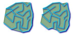
Figure 35: *ST\_ConcaveHull* over a multiline with 100% target percent (left) and 99% target percent (right) [9]
