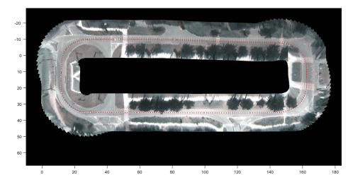
Fig. 12. Image mosaicing of the estimated path after loop closing.
