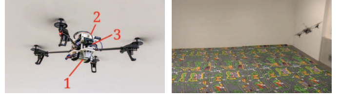
(a) A closeup of our quadrotor: 1) down-looking camera, 2) Odroid U3 quad-core computer, 3) PIX-HAWK autopilot. (b) Our flying arena equipped with an OptiTrack motion-capture system (for ground-truth recording).
