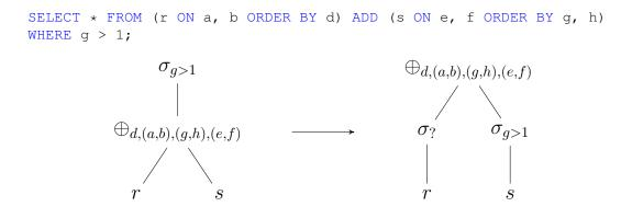
Figure 3.12.: Naive optimization of matrix addition in the relation tree
