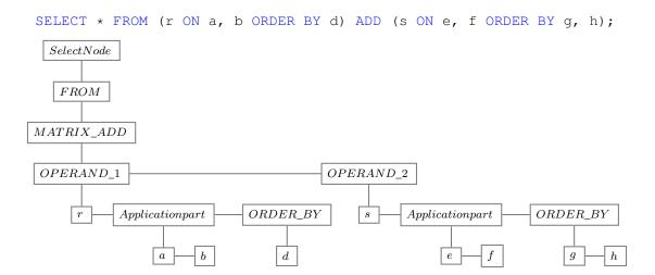
Figure 3.6.: Symbol tree for matrix addition query
