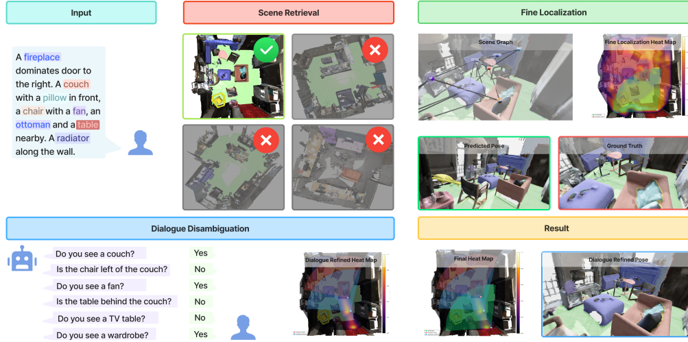
Figure 1.1: LANGLOC OVERVIEW. Input: a free-form description mentioning objects such as fireplace, couch, pillow, and fan. Scene retrieval (Section 5.4) ranks candidate 3D scenes; the correct scene (green, ✓) is identified from a pool of candidates. Fine localisation (Section 5.5) scores a dense floor grid by ray-cast object visibility, producing a heat map over candidate positions; the predicted pose (green frustum) is compared against the ground truth (red frustum). Dialog disambiguation (Section 5.6) asks targeted yes/no questions (as illustrated in the figure) and iteratively refines the posterior until it concentrates on the correct pose.
