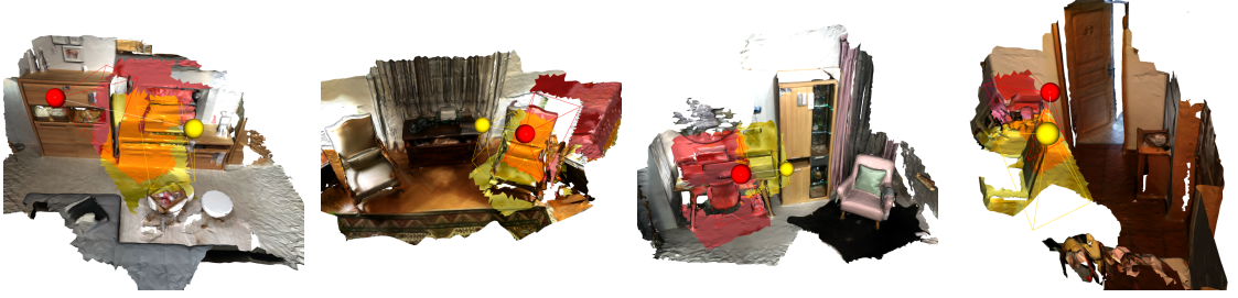
Figure 6.1: QUALITATIVE FRUSTUM OVERLAP ON 3RSCAN. Ground-truth frustum (red), predicted frustum (yellow), and their overlap (orange). The method correctly identifies both position and heading in diverse room configurations.
