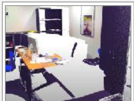
An example of the occlusions that are found in laser range scans.
