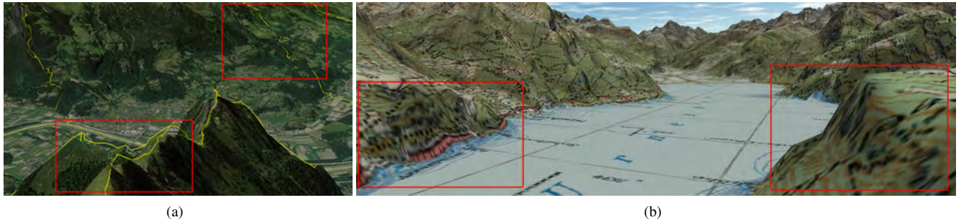
Figure 2: Example artifacts when rendering vector maps. (a) Vector lines floating or intersecting the underlying 3D terrain, and (b) texture mapping based projection and resolution artifacts.
