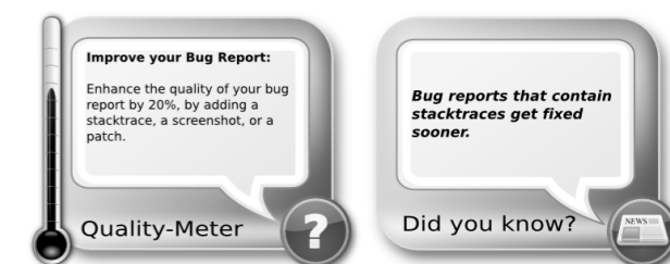
Figure 1: Mockup of CUEZILLA’s user interface. It recommends improvements to the report (left image). To encourage the user to follow the advice, CUEZILLA provides facts that are mined from history (right image).
