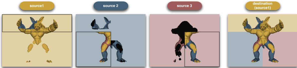
Figure 1: Sort-last rendering with direct send compositing using three channels. The first three images show the rendering buffers which contain the rendering of the partial database and the composed tile of this channel. The last image shows the final, visible destination view with the fully composited image. The channels use different clear colors to identify the tile layout.
