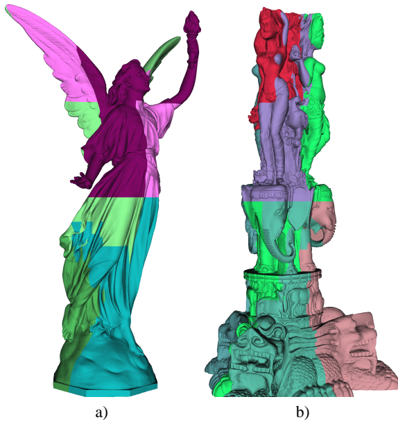
Figure 9: Destination view of the a) large and b) medium model of a six node sort-last configuration, using a different draw color for each node.
