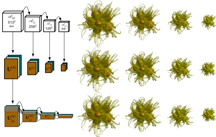
Figure 7: Factor matrix subsampling (bottom) compared to direct TA (center) derived from original subsampled datasets (top).
