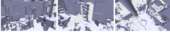
Figure 2: Indoor scans look free of noise and occlusions when seen from a viewpoint that is close to a scan position (left), but exhibit heavy occlusions and cluttering (middle, right) when the camera is moved away from such locations.
