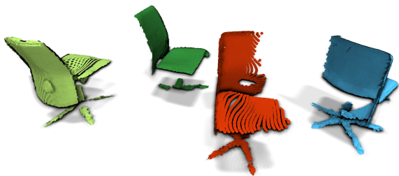
Figure 3: Multiple instances of the same chair model in an office scan (extracted with our method). Each instance suffers from undersampling and occlusion artifacts.
