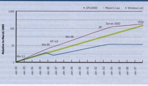
Figure 4: Windows code size (LoC) and Intel processor performance. Code size estimates are from various sources. 17-18
