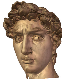
FIGURE 1. The head of Michelangelo's David statue rendered with \tau = 16 pixels screen tolerance, at 1/4 of the full resolution (510827 out of 2000606 points).
