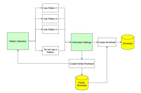
Figure 5.2: Structure of the Advanced Workload Generator
