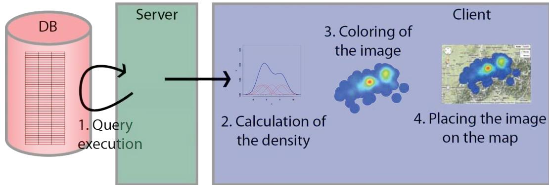
Figure 4.1: Steps of the greedy density visualization algorithm.
