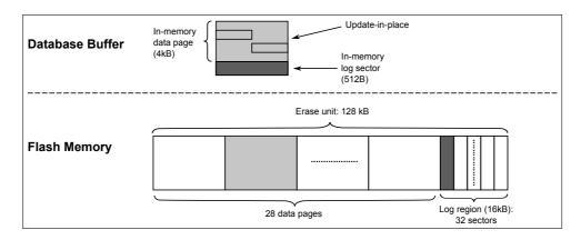
Figure 4.1: The Design of In-Page Logging
