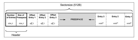
Figure 5.6: Example of a Log with 3 Entries
