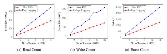
Figure 6.9: Random Read and Write: Read, Write and Erase Count
