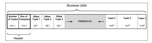
Figure 5.3: Example of a Page with 3 Tuples
