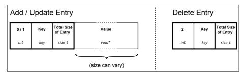
Figure 5.7: Structure of a Log Entry
