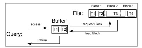
Figure 5.2: Example of a Buffer with one BufferPage
