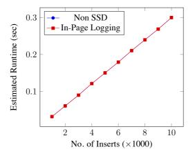
Figure 6.4: Bulk Insert: Estimated Runtime
