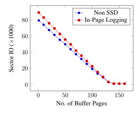
Figure 6.11: Random Block IO by Varying Buffer Size
