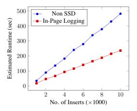
Figure 6.2: Sequential Insert: Estimated Runtime
