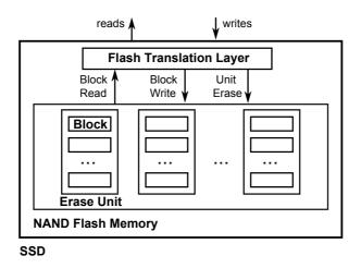
Figure 2.1: Simple Design of a Solid State Drive
