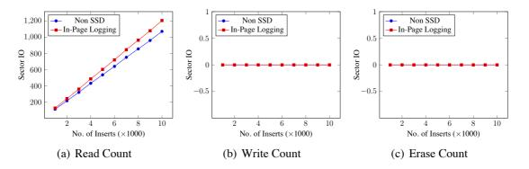
Figure 6.7: Sequential Scan: Read, Write and Erase Count
