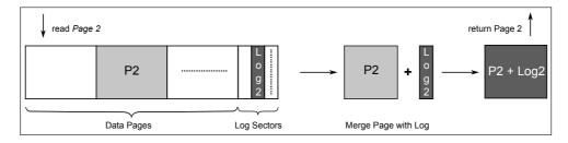
Figure 4.3: Read a Page with corresponding Log
