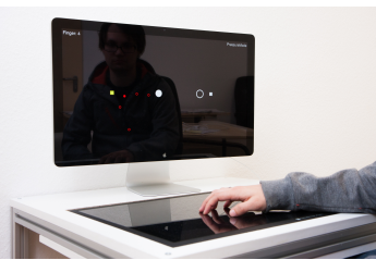
Figure 1: Indirect multitouch setup: horizontal surface for expressive input, vertical surface for ergonomic display.
