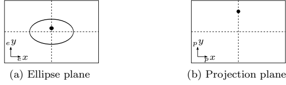
Fig. 3 Considering C in Fig. 1 as the camera view point. Contour of the outer circle with the appearance of the circle's centre point (Fig. 3a) and the position of the centre point in the projection plane (Fig. 3b).
