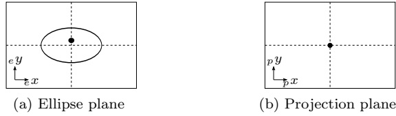
Fig. 5 After applying R_a the ellipse in Fig. 5a has its desired shape and orientation. But the optical axis goes still through the centre of the appearance (Fig. 5b). A rotation R_b forces the centre to appear in the desired position showed in Fig. 4b.
