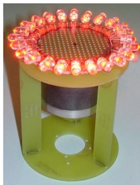
**Figure 4:** The circular set of LEDs forming the light source, positioned on the mirror.
