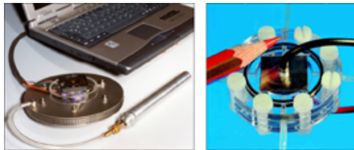
Fig. 2.2: Fuel cells developed by Fraunhofer ISE. Left: fuel cell powering a notebook. Right: a tiny fuel cell for use in applications such as cellular phones.
