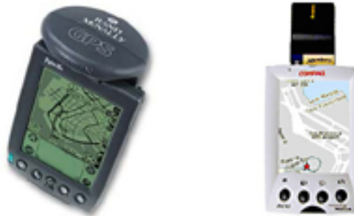
Fig. 4.3: Left: Clip on system “StreetFinder GPS” for the Palm III from Rand McNally; Right: Pretec’s CompactGPS, a GPS sytem on CompactFlash card.
