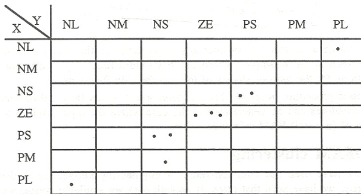
Figure 7.16: Distribution of the quantization vectors, given the data shown in figure 16.
