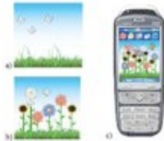
Figure 1. UbiFit Garden's glassable display. (a) at the beginning of the week—small butterflies indicate recent goal attainments, the absence of flowers means no activity this week. (b) a garden with workout variety. (c) the display on a mobile phone—the large butterfly indicates this week's goal was met.
